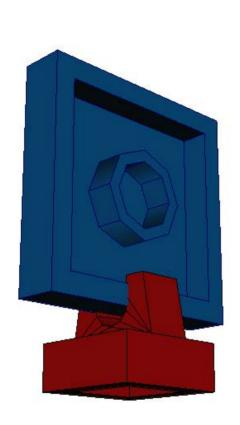
All are illegal because the receiving brick has smaller dimensions than the one being connected to it.
