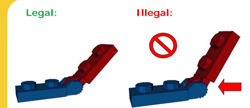
Click hinges must be in 'click.' Approved angles are in multiples of 22.5 degrees. Some LEGO projects require an engineer to determine whether an angle is legal.
