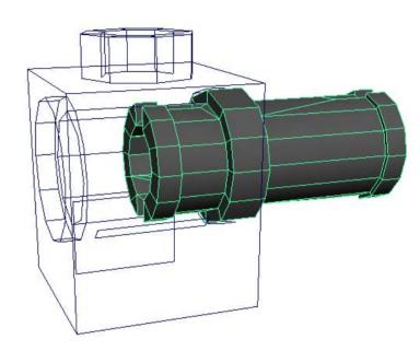
Both ends of a Technic hole are larger than the diameter in the middle. Until it 'snaps' into place, the half-peg is in compression and could be permanently damaged over time. Also, by not being locked into place, the element can easily pop out during play.
