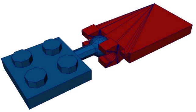
Not recommended because the two plates will not be at the same height. This causes the assembly to be 'out of system.' Also, there are other elements in the assortment that can accomplish this legally.
