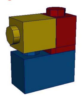
The word *LEGO* molded onto the studs of most System elements increases the height of the stud by 0.14mm. This extra height causes the stud on the blue brick above to touch the side of the yellow one.
