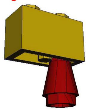
Because there is no stop at the top of the cone, the red element could be pushed in too far. This will stress the pin and inner walls of the yellow brick
