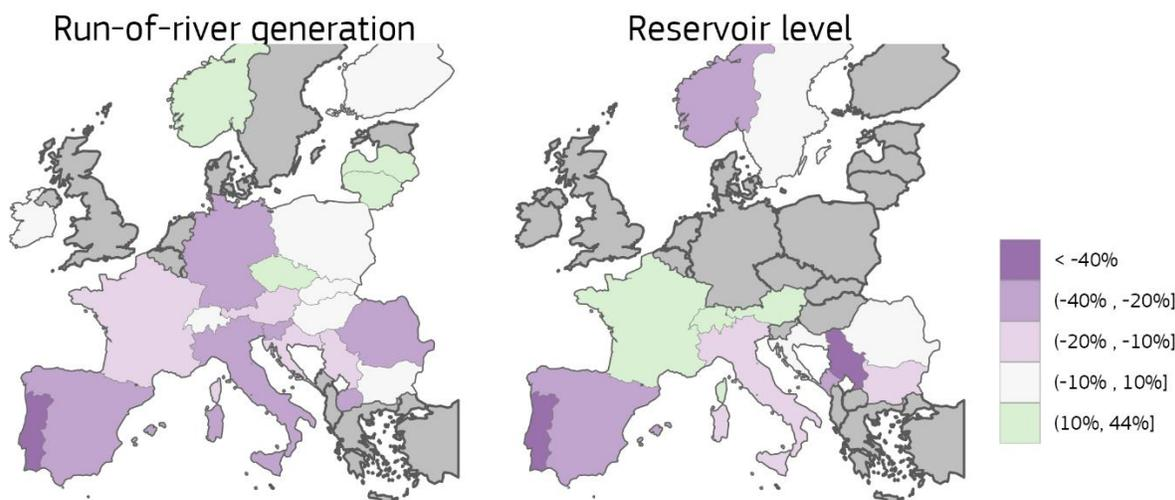
**Figure 12:** Percentage difference between the cumulative hydropower run-of-river generation and storage levels for the week 14 of 2022 compared to the same week in the period 2015-2021. Data from the ENTSO-E Transparency Platform (retrieved 20/04/2022).
