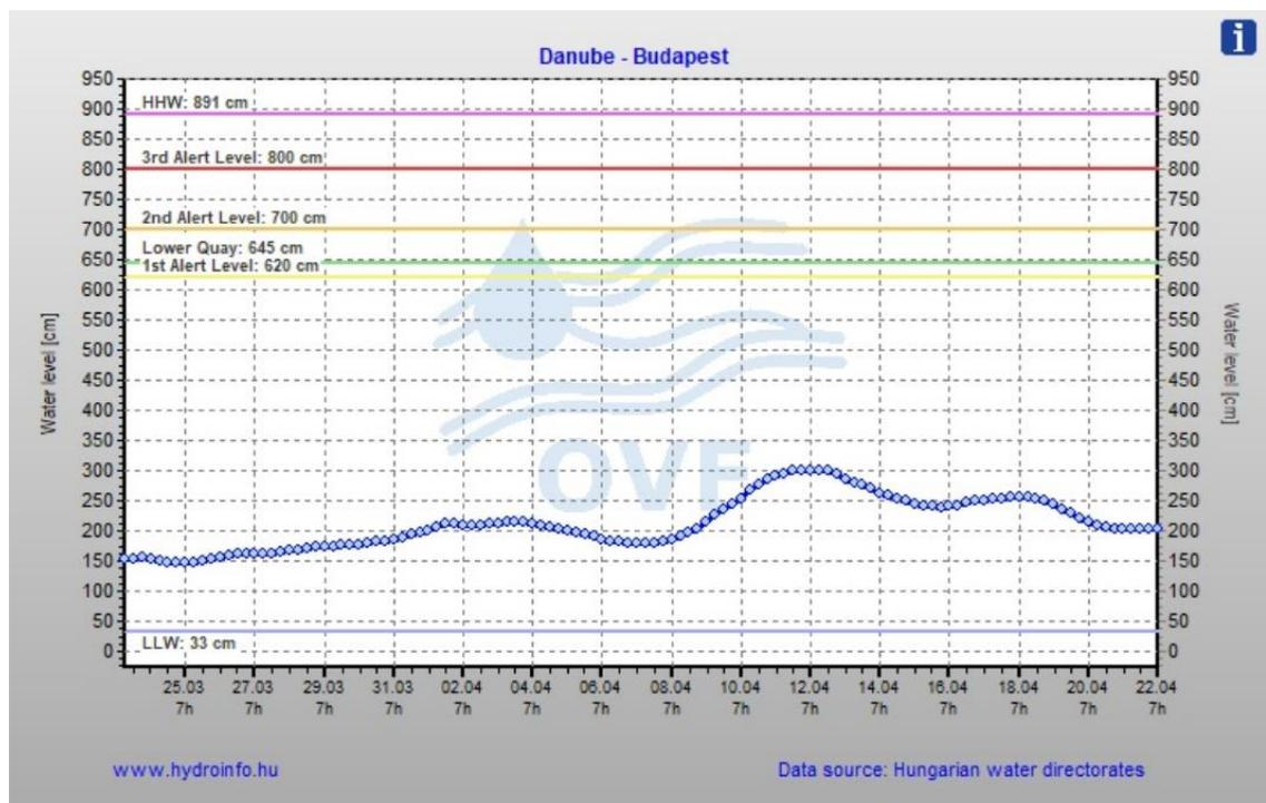
**Figure 6:** Water level time-series of the Danube (Budapest) from 25<sup>th</sup> March 2022 to 22<sup>nd</sup> April 2022. Source: Hungarian Hydrological Forecasting Service (<https://www.hydroinfo.hu>)
