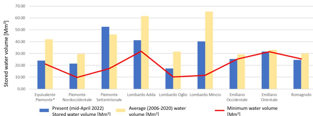
**Figure 14:** Cumulative stored water volume at mid-April 2022 (blue bars), average stored water volume for the same period (2006-2020, yellow bars), and historical minimum volume (red line) for mountain reservoirs for, each sub-basin of the Po basin from west to east, source to outlet. Source: Permanent Observatory on water use - Po River District Basin Authority.
