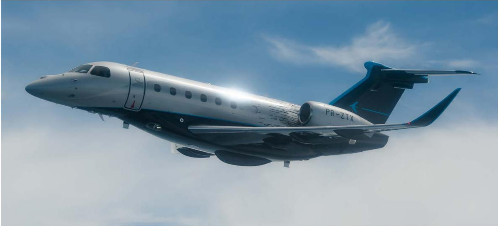
Camelier who developed the flight controls tells me that wing reinforcement because of such large winglets was not needed thanks to a «load alleviation» function. It was designed to reduce the stresses applied to the wings during high-speed turns using simultaneous aileron deflection upwards of  $10^\circ$  during those turns.
