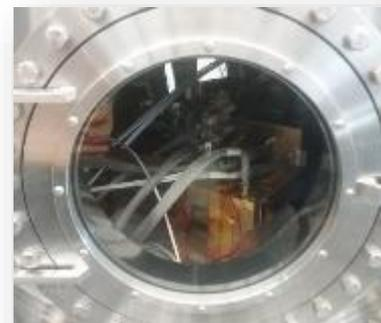
Thermal vacuum testing of RP subsystems
